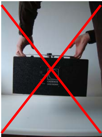
Photo 2: do NOT lift the Okki Nokki by the turntable
