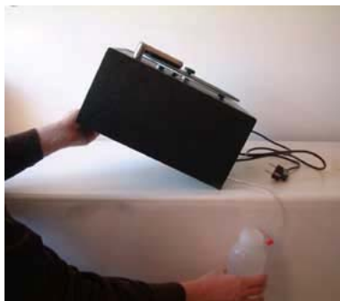
Photo 6: draining the cleaning liquid
